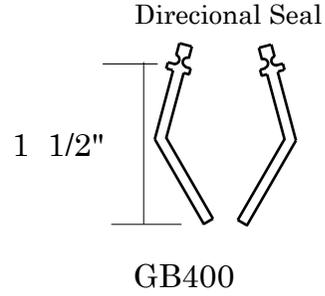
Choose the Holding Frame Style and insert the Rubber in the direction to solve the problem
